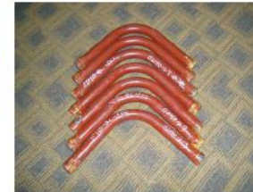
Final SH bends 未过弯头
